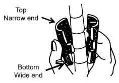
NOTE: The smaller end on the snap sleeve is the top. Be sure the smaller end on the sleeve facing up.
