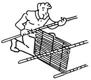
NOTE: The shelf should lock with posts without extra tools. If it's difficult to assemble, check openings and make sure they have locked properly.
